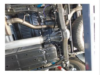
**Step 5**: Next, attach the Overaxle pipe to the muffler Assembly using the supplied 3.00" clamp and fit the hangers.
