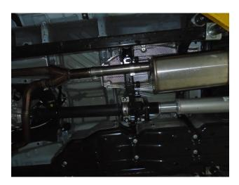
**Step 3:** At this point if you are installing the MagnaFlow exhaust system on a Long Bed vehicle you will need to add the 15" Extension Pipe using the supplied 3.00" clamp. (The short bed does not require this pipe).
