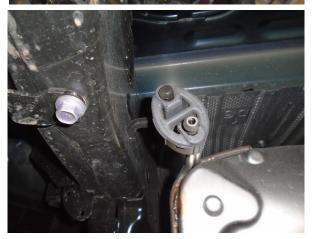
**Step 1:** To remove the OE exhaust system, loosen fasteners at the inlet flanges (2) where they connect to the catalytic converters. Working front to rear disengage the hangers from the rubber insulators, remove the remaining fasteners at flange junctions and drop the system. (Retain the Inlet fasteners, gaskets and rubber insulators as they will be used to install your new system.)
