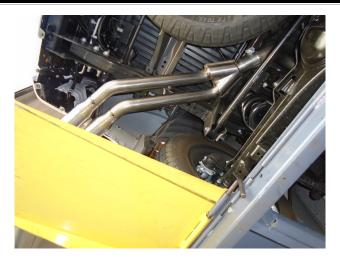
**Step 6:** Finish the installation by attaching the Tail Pipe Asembly to the Over Axle Pipe using the supplied 3.00" clamp and fitting the hanger into the rubber insulator.
